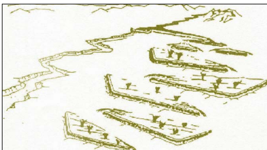
Flood Water Diversion and micro-catchment basins
