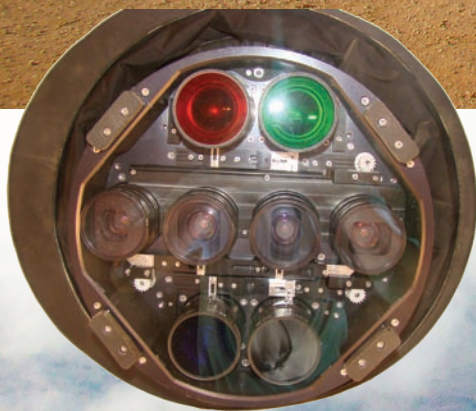
Vexcel UltraCam-X 196 megapixel large format aerial camera with processing equipment
