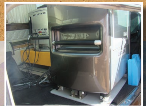
Kamerada dayaaradda oo leh qalab wax lagu hagaajiyo oo qaab weyn oo ah Vexcel UltraCam-X 196 megapixel
